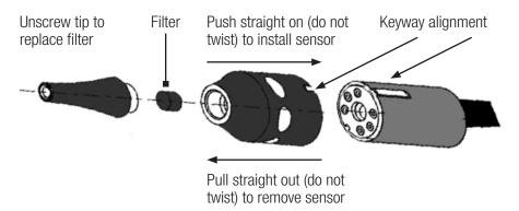
**IMPORTANT:** The instrument's software is designed to alert the user if the sensor is dislodged or defective. If the sensor is not fully inserted into the six-pin socket, or if it is defective, the instrument will not come out of the "Warm Up" mode for proper operation when the power button is turned on. Additionally, if the instrument becomes unstable during its operation, it is an indication that the sensor may be defective or dislodged.
